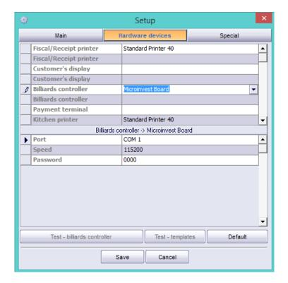
When selecting a particular device model from drop-down menus, the program automatically displays the settings that are configured by the manufacturer and are necessary for the proper functioning of this device. Note that these settings can be changed, if it is necessary. *Save* button keeps the made changes and close the window and the button *Cancel* (or Esc on the keyboard) closes the window without performing a record.
